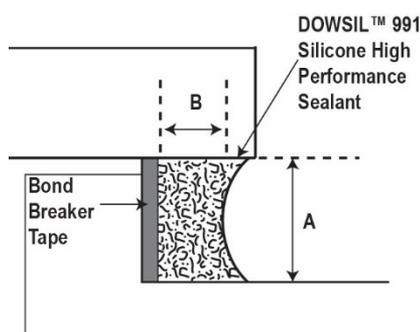
Open-cell polyurethane foam, closed-cell polyethylene or non-gassing polyolefin are the recommended backing materials for most joints; use polyethylene tape for joints too shallow to allow backer rod (see Figure 2). These materials permit application for a thin bead and act as bond breakers, which allow the silicone sealant to move freely with the joint.
